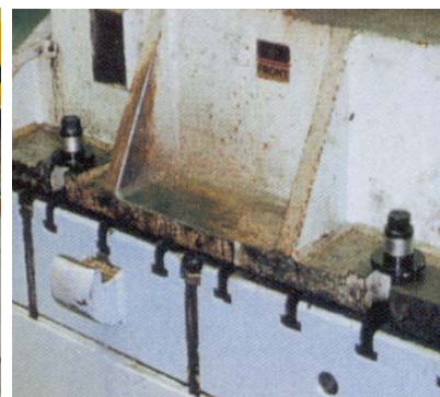
MC-Clamp for lower die, in clamped position
