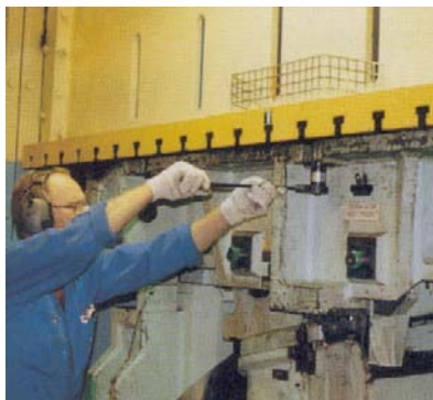
MC-Clamp in clamped position
