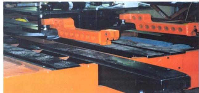
Domino cart with bridging arms for space between press table and cart
