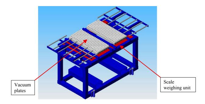
Data for weight of the panel is stored in the control system.
