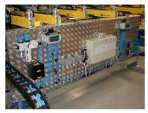
Option: Absolute Encoders for indication of the Fanning magnet position. Data is stored in the control system.
