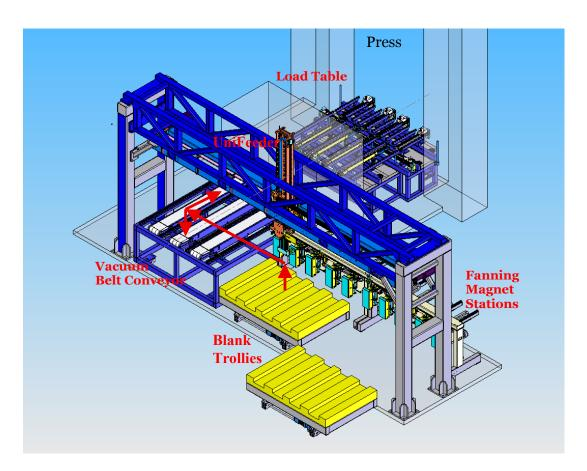
The UniFeeder picks up one blank at the time, from eighter of the two pick-up stations and brings it to a leave position, in the show case a Vacuum Belt Conveyor. The conveyor moves then the blank to the Load Table for centering before it is loaded into the press.
